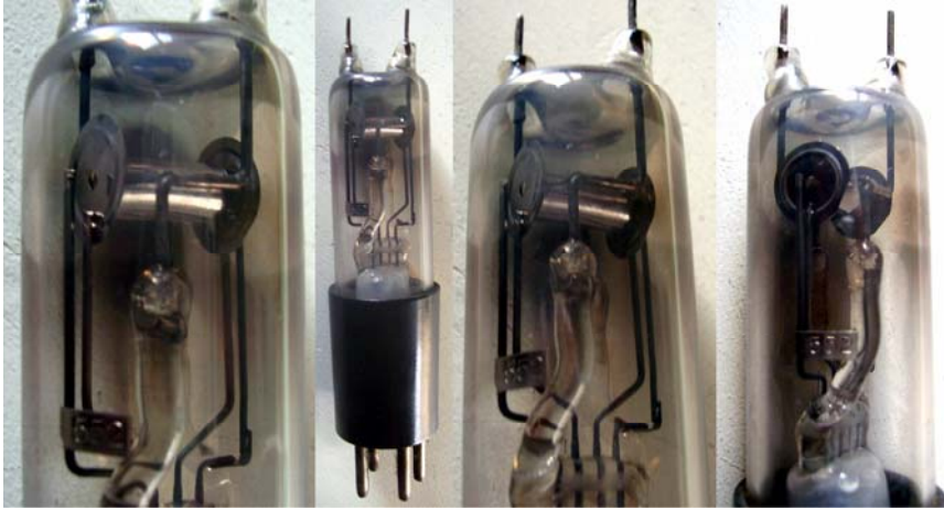
Midget split-anode magnetron probably used for early Megaw's experiments around 50 or 25 cm.
