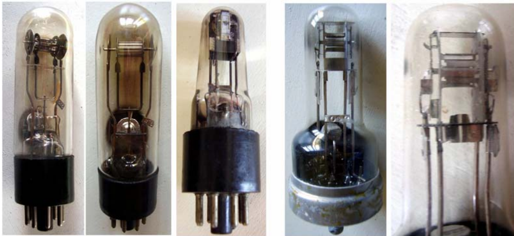
Three GEC 'squirrel cage' magnetron prototypes built during the development of CV79 and CV89, the last two samples in the image. These were used in the Wireless Set No. 10, operating at 7.5 cm. The prototypes could be dated from the late 1940 to 1942. The set, designed by Megaw and Willshaw, became fully operative from 1944.
