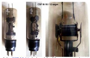
Gutton's 12-segment variant of the <u>CSF M-16</u>, designed for Megaw to experiment with behavior in the different oscillating modes, according to module 12, module 6 and module 3.
