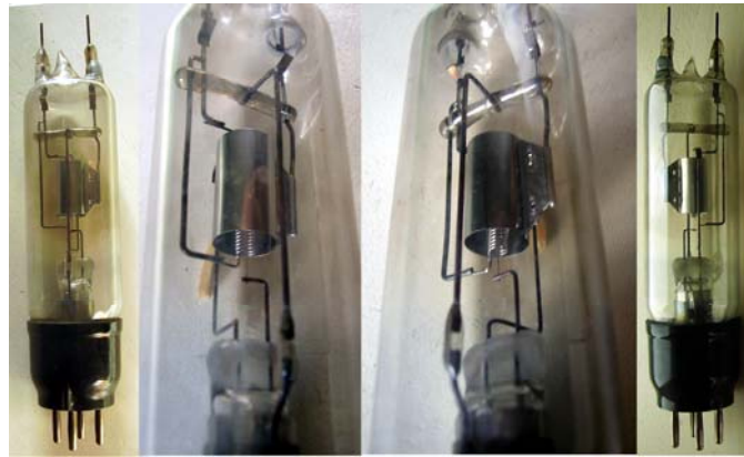
Early gridded magnetron , the grid being a spiral wire surrounding the filament. Its vertical electrodes and the use of glass spacers to hold them in place suggest a 1935 design.
