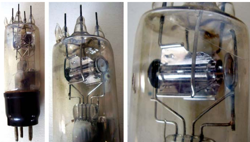
A laboratory sample of the E880/NT75 four-segment magnetron designed for the British Admiralty by Megaw at GEC Wembley. The NT75 was used in the transmitter of a ship-to-ship secure communication set described by the same Megaw in a 1947 paper.
