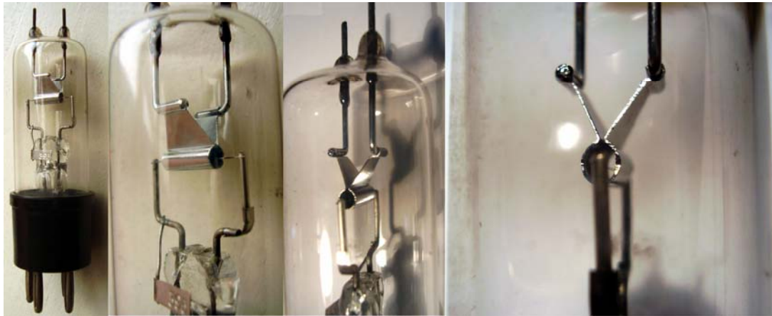
A tiny spit-anode magnetron with internal back loop . It could apparently operate at very high frequencies, probably at 10 cm (3 GHz).
