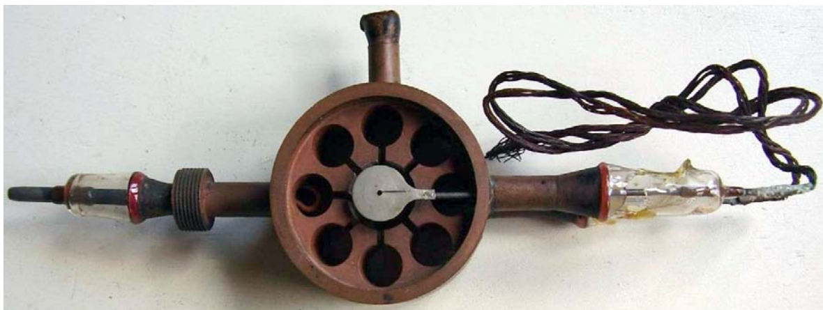
The very early GEC laboratory prototype of the British cavity magnetron , July 1940.
