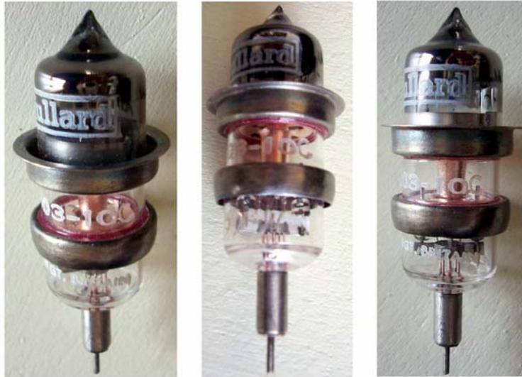
Disc seal planar triode without internal feedback, intended for use in common-grid, grounded-anode coaxial oscillators or as power amplifier.
