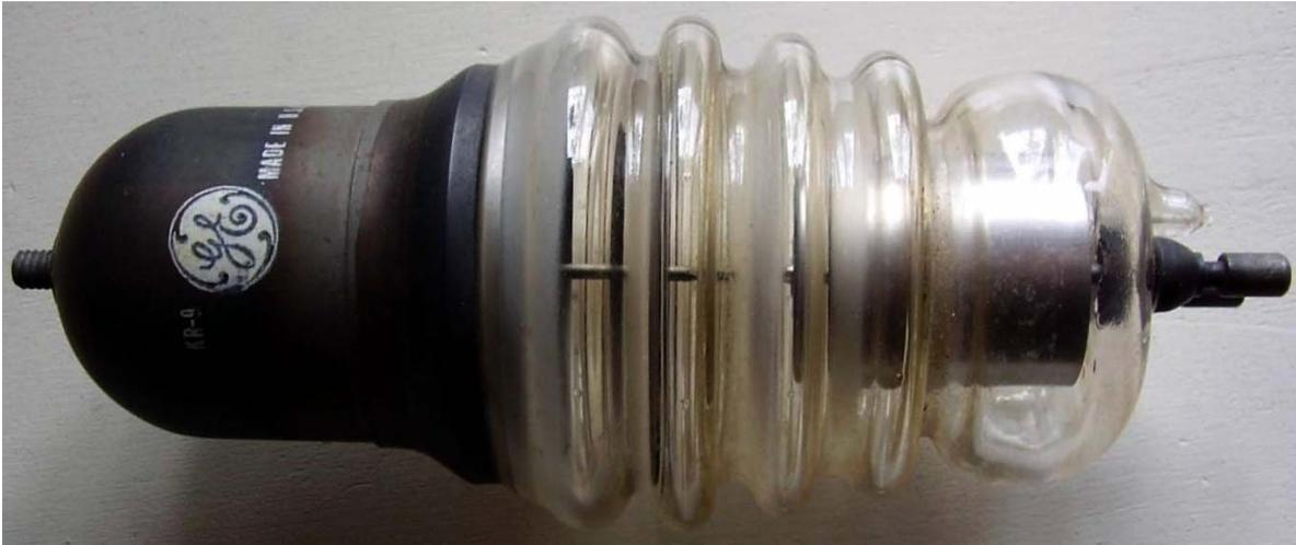
General Electric high voltage rectifier for X-ray applications. Intended to be mounted in any position, only supported from the anode. High-emission thoriaed-tungsten filament.
