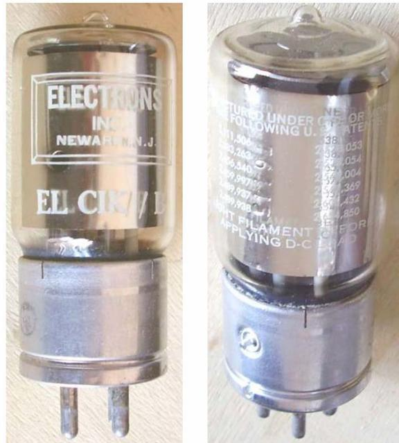
Xenon triode thyatron; 2 kV PIV, 1A; 25 sec heating time minimum.
