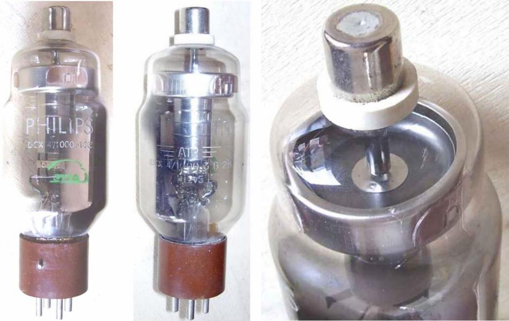
Xenon rectifier. Wide temperature range replacement for 866A.
