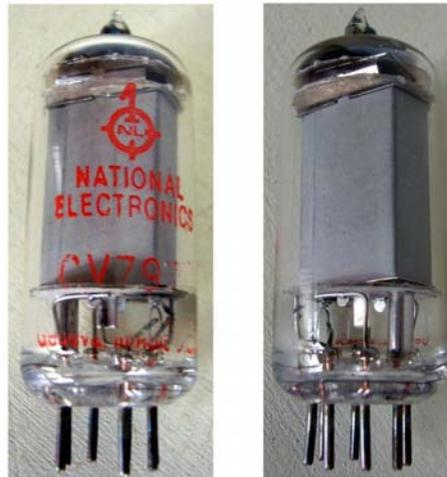
Miniature thyatron tetrode, British equivalent to [5727 / 2D21W](#). General purpose applications, including relay, grid-controlled rectifier, pulse modulator, clock generator and even gas noise generator.
