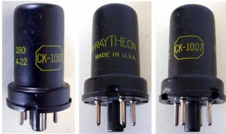
CK-1007 is a gas-filled rectifier intended for vibrator B+ supply circuits in car radios and other mobile equipment operated from storage batteries.
