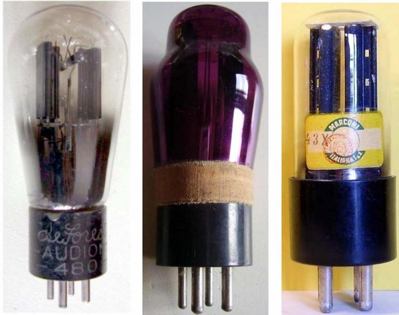
One of the most used vacuum rectifier from 1927 well into the fifties. Known as 80, 180, 280, 480 and many other names, depending upon their manufacturers, it was produced with a variety of bulbs, from the ballon type to ST and even tubular, GT-like, versions.
