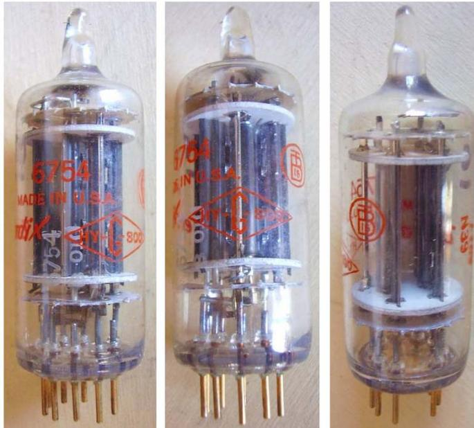
All-glass high-rel miniature 9 pin rectifier. Also known as TE-36, equivalent to Western Electric 412A.
