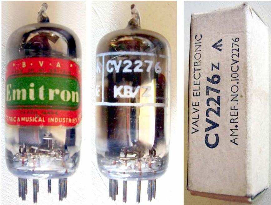
High-gain VHF pentode, incorporating a single stage secondary emitter to increase gain. EMI also registered the tube in America in October 1953 as 6351, RMA record [1250](#). Equivalent to the commercial Marconi [Z319](#), Nov. 1954.
