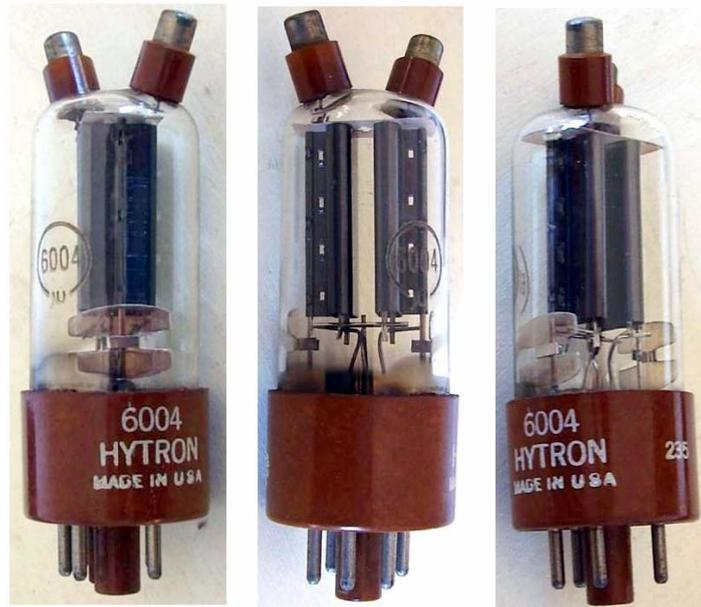
High-rel full-wave rectifier derived from 5Y3. Plates connected to the two top caps, seating on low-loss phenolic spacers for improved insulation. 90,000 ft. altitude.
