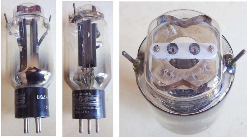
High-rel, high altitude (60,000ft) version of 1641, full wave rectifier. Side plate contact pins for improved insulation.
