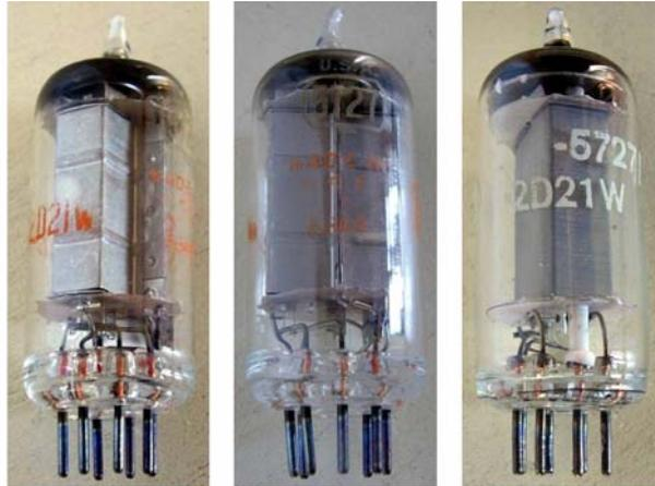
2D21 is a miniature thyatron tetrode, all-glass version of [2050](#). General purpose applications, including relay, grid-controlled rectifier, pulse modulator, clock generator and even gas noise generator. Also made in the hi-rel version 2D21W, registered as 5727. Equivalent to British [CV797 / EN91](#).
