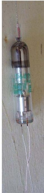
High-voltage diode used for high-voltage CRT circuits in oscilloscopes. Subminiature body, flying leads.
