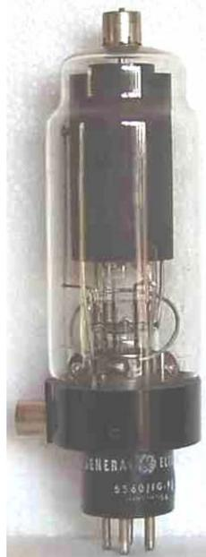
Mercury tetrode thyatron, grid from the side of the base. 1.5 kV PIV, 2.5A.
