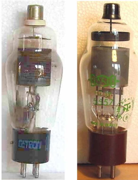
Mercury-vapor industrial thyatron. Grid-controlled version of 866A.
