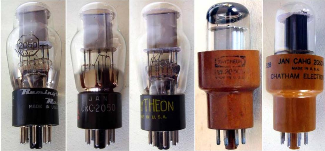
Gas thyatron, xenon filled. 1.3 kV PIV, 100mA average. 2051/VT-109 is a slightly derated version, replaceable by 2050.
