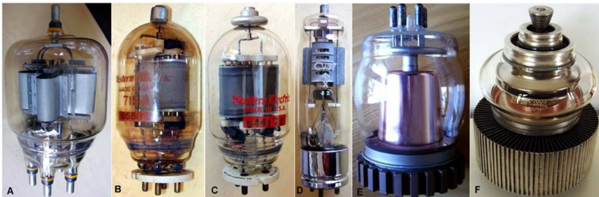
Fig. 7.1.6 - Vacuum tubes designed to operate as power switches in pulse modulators. A) Western Electric 701A was hastily designed to drive the very early WE magnetron, the 700A. The required emission was obtained assembling four electrode sub-systems of the 350A power tetrode, cathode and grids, inside a cruciform plate. Grids were gold plated to decrease secondary emission when pulsed positive. B) 715A was an evolution of 701A for airborne applications. Here the four cathodes were placed side-by-side into a single plate and grid system. 715A evolved through several steps, with improvements of grid cooling and of the insulation. C) 5D21 was a further evolution during the war of 715B, with the addition of a top guard ring to prevent corona discharge at high altitudes. D) CV57 was a quite small British tetrode capable of handling 5 A pulses at 11 kV. E) Amperex AX10318-1 is a tetrode intended to operate immersed in oil to switch 5 A at 100 kV. F) ML-7003 was a screened grid triode used in pulse modulators up to 2.5 MW. It was rated for operation as switch at 40 kV, 80 A.
