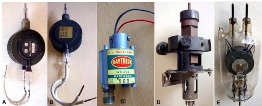
Fig. 6.3.9 - A) CV1479 to CV1482 replaced CV76A to CV76D. 450 kW out pulses. B) MC86 was a French CSF magnetron. C) OK698 was a tiny magnetron for beacon transmitters. D) OK174C is a rare sample of FM modulated magnetron intended for microwave television relays. It uses six auxiliary electron guns directed toward the resonators in order to modulate the generated frequency. E) Brown Boveri MD10/2000 Turbator includes a coaxial resonator. (Click on image to enlarge)
