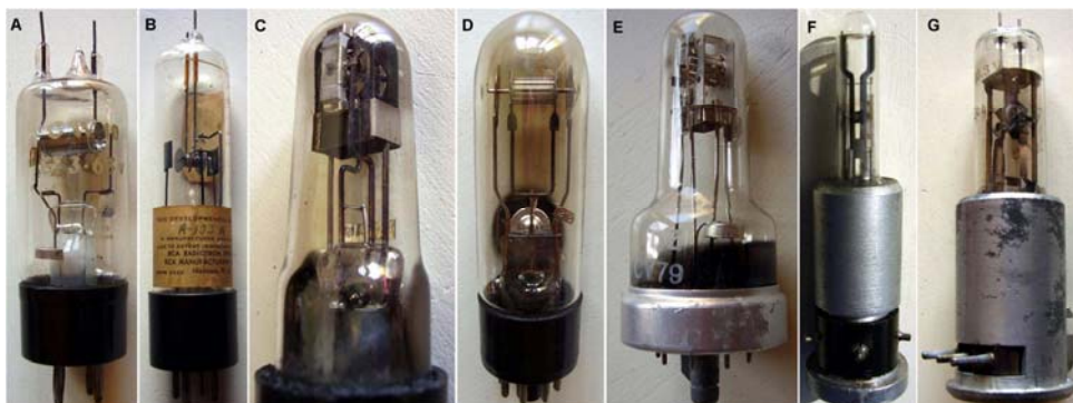
Fig. 6.3.5A - Low-power CW magnetrons. In these tubes anode is split in two half sections or even in fingers, alternately connected to one of them. A) British CW10 is a rare split-anode magnetron which can be dated around 1935. Used in the very early experiments on UHF radio-localization. B) RCA A-103A is a very rare prototype of split-anode magnetron with self-contained resonator, operating around 3 GHz. C) GEC interdigital 8-segment prototype. D) 12-segment GEC interdigital prototype. E) CV79 was one of the British interdigital types in production late in the war for use in a microwave relay system. F) German RD2Mh was a small-power magnetron, 300 mW around 5 GHz, used in microwave test generators. G) German RD4Ma delivered 12 to 15 W at frequencies around 1.5 GHz. It was used in a microwave communication link. (Click on image to enlarge)
