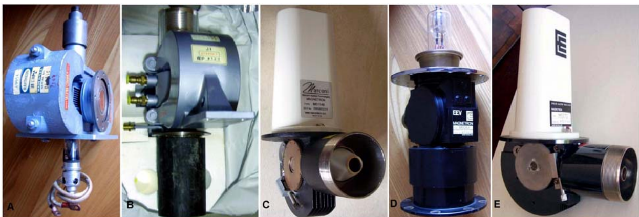
Fig. 6.3.10 - High-power magnetrons. A) 6344A is a C-band magnetron capable of generating 260 kW output pulses. B) 6410A is one of the most powerful magnetron for early warning radars, 5 MW out pulses for a weight exceeding 26 kg. This sample was made by Italian ELTEL, under Raytheon license. C) British Marconi M5114B was a tunable S-band magnetron, 1 MW out pulses. D) M5125X is a 2 MW magnetron used in linear particle accelerators, LINACs. E) M5170 is a British EEV 1 MW tunable magnetron. (Click on image to enlarge)
