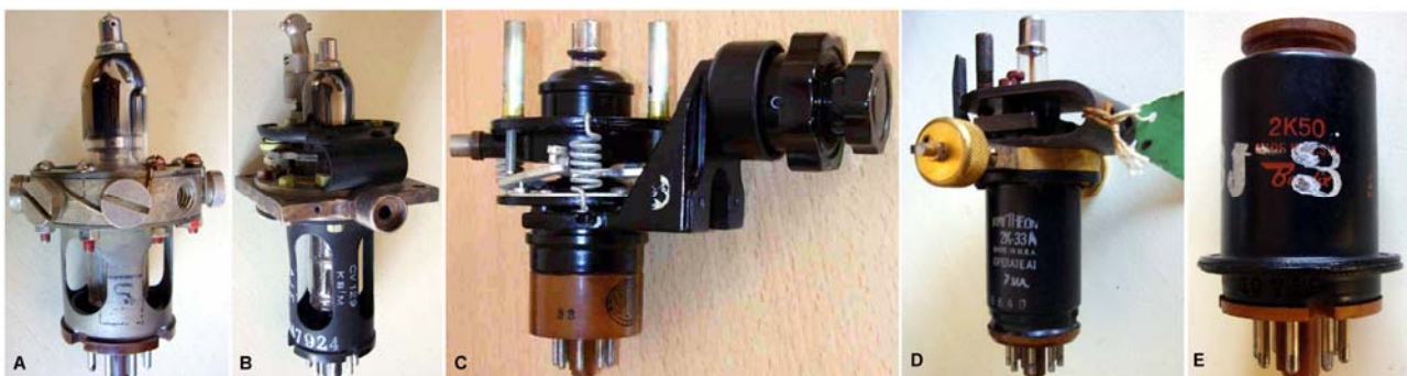
Fig. 6.2.4 - More klystron tubes developed during WWII. A) CV238 , capable of operating at 250 volts, was introduced in 1943 to replace high voltage types, as CV35, in airborne applications. B) CV129 , a British X-band klystron, was readily phased-out in favor of 723A/B. C) 2K41 was one of the many klystron devices designed by Sperry during the war. D) 2K33A , the first K-band klystron, was the result of a design performed in England at Clarendon and perfected in America by Raytheon. E) The electronically tuned 2K50 was the refined WE answer to 2K33. (Click on image to enlarge)
