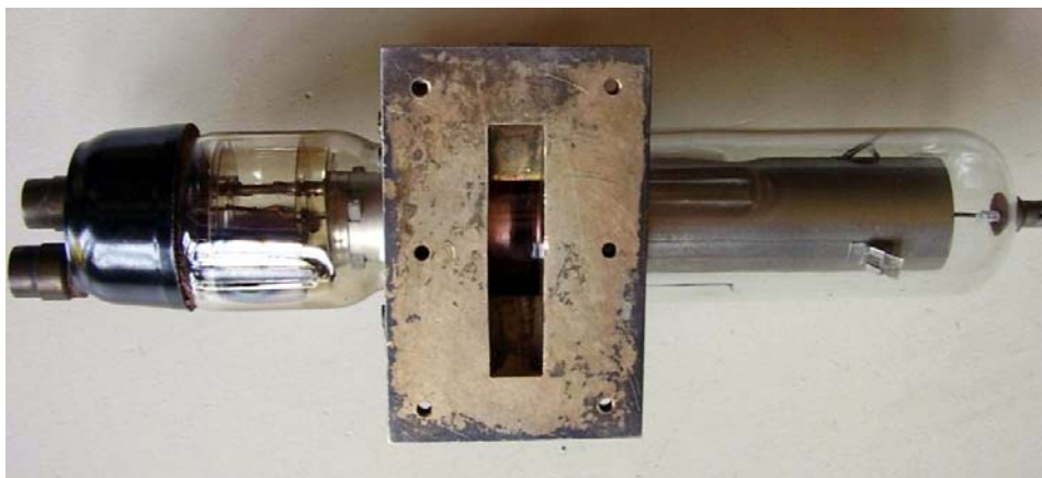
Fig. 6.2.9 - The collection includes a rare sample of British EMI CV150 , the only S-band power klystron intended to replace magnetrons as pulsed oscillator in airborne radar sets. Click on image to enlarge.
