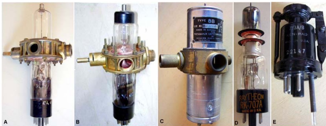
Fig. 6.2.3 - British, Canadian and American klystrons used as local oscillators in the early S and X band radar sets. A) CV35 was one of the early British klystrons used since 1941 as local oscillator in S-band radar sets. It replaced the developmental type NR89 or ‘Sutton tube’ by the name of its designer. B) CV67 was a frequency variant of CV35. C) Canadian REL 8B was presumably derived from the NR89 Sutton tube, by adding a metal shield and a 4-pin base. D) The WE 707A was the very early American design of an S-band klystron in WWII. Its efficiency was quite poor and the grids became almost white in operation. D) 723A and the improved 723A/B were the early X-band reflex klystron designed by Western Electric before the 2K25. (Click on image to enlarge)
