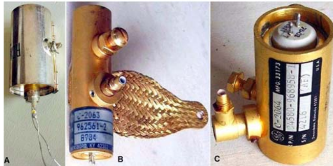
Fig. 5.17 - Microwave modules. A) RCA 6562 was a module designed for radiosonde transmitters at 1680 MHz. It used a pencil tube as oscillator. B) General Electric C-2063 was a Microwave Circuit Module, MCM, intended as local oscillator in radio-altimeter receivers. 4300 MHz center frequency. C) GE C-2064 was the transmitter MCM companion of C-2063. 4300 MHz center frequency, 70 W peak power. (Click on the image to enlarge)
