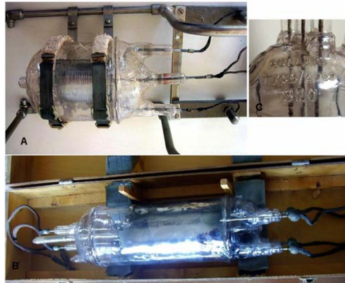
Fig. 4.2 - Due to the high melting temperature of the envelope, silica valves were relatively small, their diameter just being slightly greater than the plate diameter. A) NT45A was a quite small transmitting triode, rated for 1.25 kW power dissipation. B) TYS 5/2000 , rated for 2 kW dissipation, is 477 mm long. C) Close-up view of the hand made writings in fused silica. More silica valves are in the radar dedicated tubes. Click on the image to enlarge.
