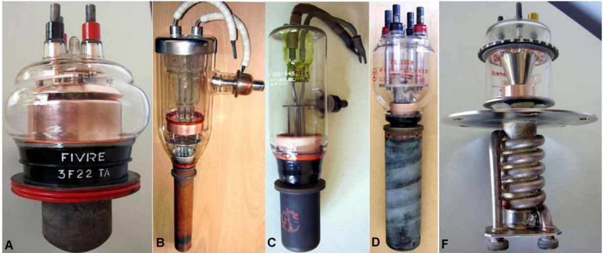
Fig. 4.4 - Water-cooled transmitting tubes. A) The Fivre 3F22-TA / 5771 is an improved version of the folded anode 880 , 22.5 kW. B) VT-34 / JAN-207 is rated for 10 kW anode dissipation. C) The smaller 846 was rated for 2.5 kW. D) The heavy 5668 was capable of dissipating 20 kW through an external water jacket. F) The integral jacket Amperex 8592 was rated for 6 kW anode dissipation. (Click on the image to enlarge)
