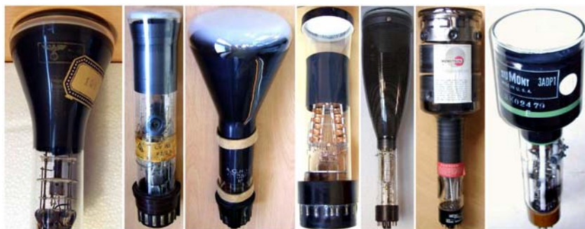
Fig. 10.3 – Some of the CRTs in the collection, starting from WWII. Also included dual-beam, distributed deflection, and memory types.
