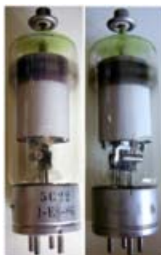
Fig. 2 - An ELSI 5C22 with the EIA standard code and a puzzling suffix, J-ES-SG, which appears to be a JAN qualified manufacturer code. Maybe that ES stays for European Supplier but this is just a guess. Click on the image to enlarge.
