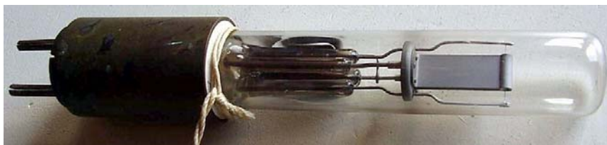
Fig. 7 - Siemens RM4025 looks to be a split-anode magnetron with self-contained resonating system. It was designed for operation at 3 cm. Still in evaluation phase at the end of the war. Click on image to enlarge.
