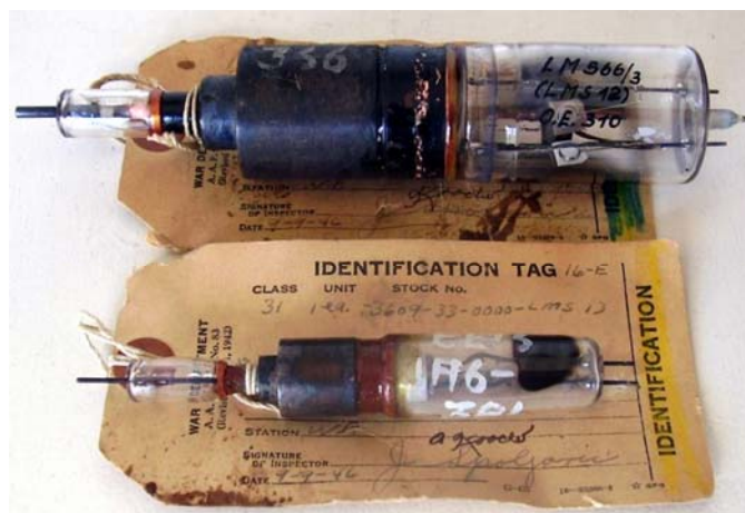
Fig. 3 - Although LMS12 and LMS13 have the same shape, their size is considerably different. Few doubts that LMS13 was readily designed as scaled down version of the LMS12. Click on image to enlarge.
