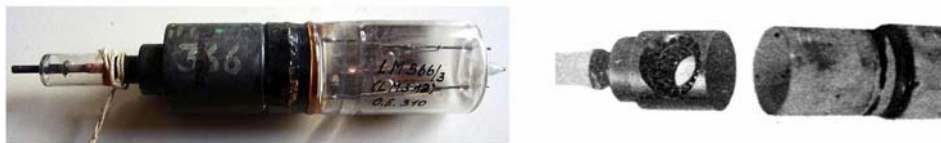
Fig. 2 - Left, the external shape of the LMS12, the thick coaxial probe pointing to left. Right, construction details of the new family of German magnetrons: the sleeve, sealed to the bottom glass body with cathode and heater leads, is brazed around the anode block. Click on image to enlarge.
