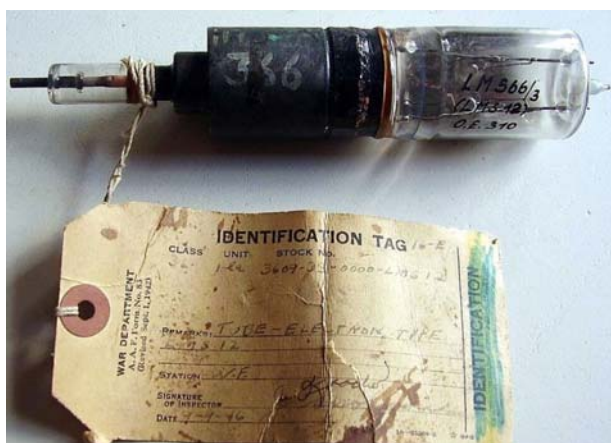
Fig. 4 - This is the only known sample of LMS12 still existing today. On the glass bulb also its experimental code, LM 566/3, is well visible. It still retains the US War Department classification tag, dated 1946. The rod on the left looks to be the center conductor of the coaxial output. The two heater/cathode pins are on the right of the large glass bulb. Click on the image to enlarge.
