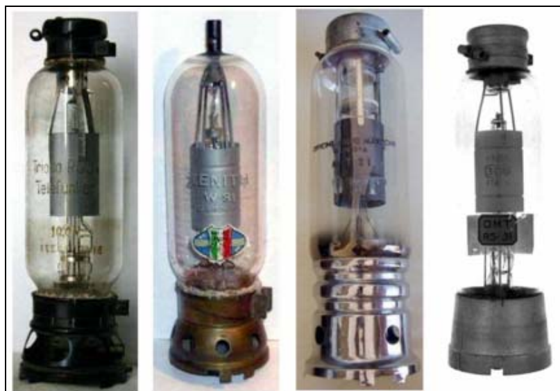
Fig. 7 - Look of the four different versions of the German RS31g made in Italy by Telefunken, Zenith (Philips), Marconi Genova and Fivre. (Click to enlarge)
