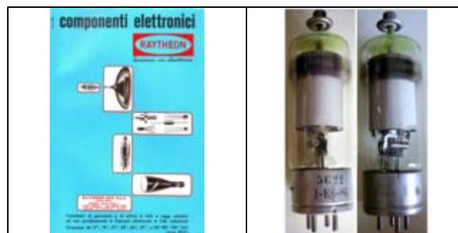
Fig. 8 - Left, a Raytheon-Elsi ad, showing the wide range of commercial and industrial products offered. Right, two views of an ELSI 5C22 hydrogen thyratron NATO qualified. (Click to enlarge)
