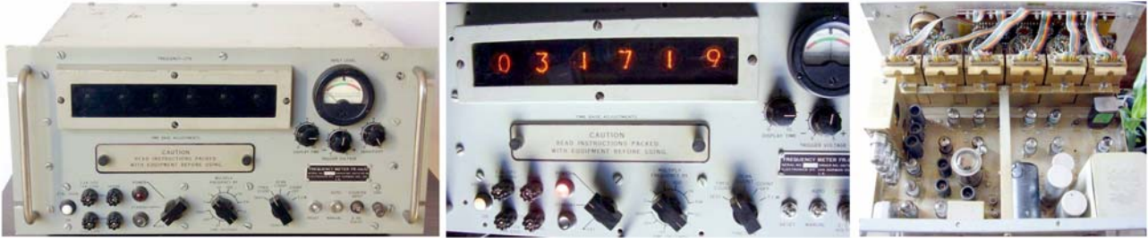
Fig. 10 – Pictures of the FR-114U frequency meter.
