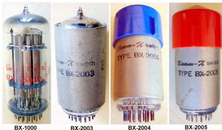
Fig. 7 – The unshielded BX1000 and of some shielded Beam-X types.
