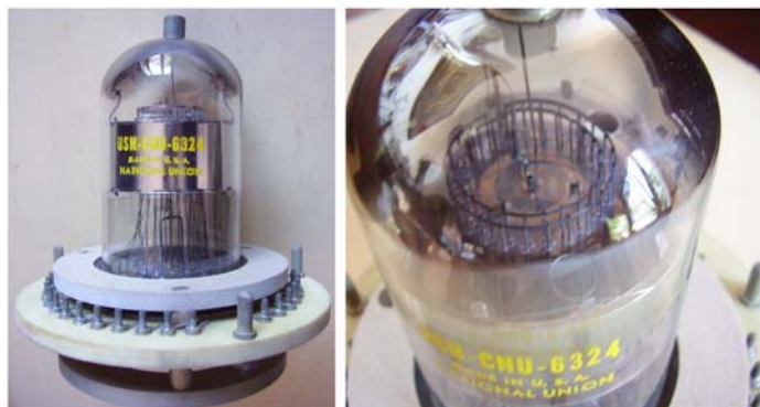
Fig. 1 – The National Union 6324 intended as 25-line multiplexer.
