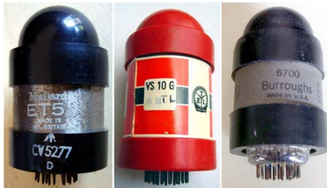
Fig. 8 – The Mullard ET51 and the VS10G compared with the Burroughs 6700.
