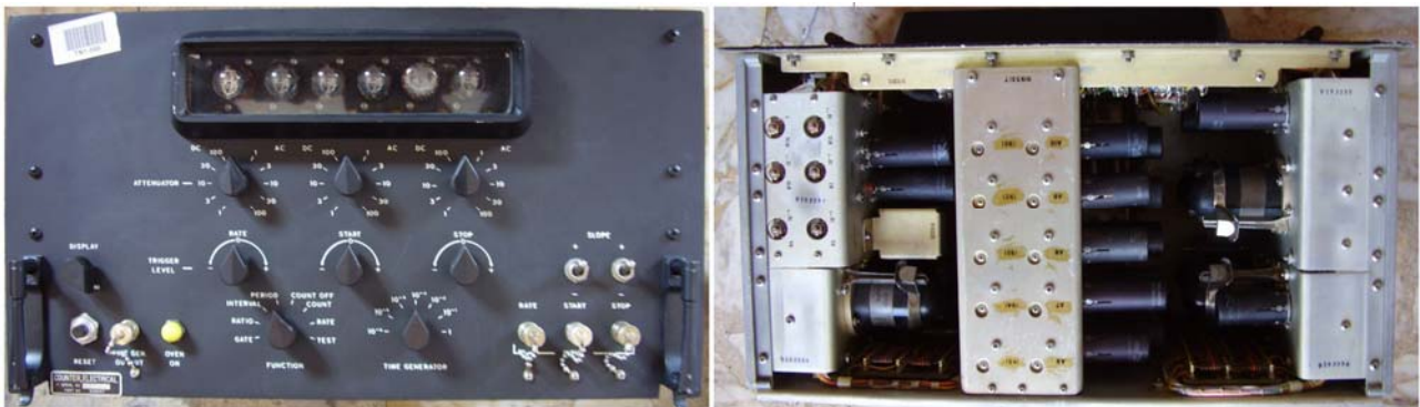
Fig. 14 – Pictures of the 6-digit trochotron counter, probably from rangekeeper set.
