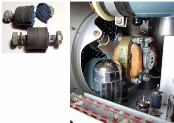
Left, a broken rubber spacer and a good one. Right, the fan just serviced.
