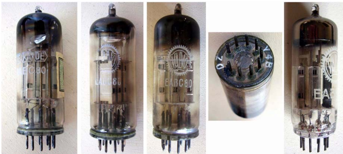
Fig. 3 - Samples of very early European EABC80s. The first one is branded TeKaDe while the second and the third ones are branded Valvo. Anyway all have an Y4B short code printed on the base and probably were pumped at the Mullard Blackburn plant in England. In the three samples above the base is glazed to the envelope by low temperature sealing process and the electrode assembly is held rigidly by a couple of rods well visible in the first photo, no need for mica spacers. The last sample on the right is the normal miniature version.
