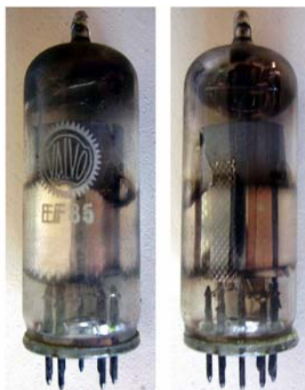
Fig. 6 - Two images of an early glazed EF85. According to the short code stamped on the base, Y3A, this sample was probably pumped at Wiener Radio Werke.
