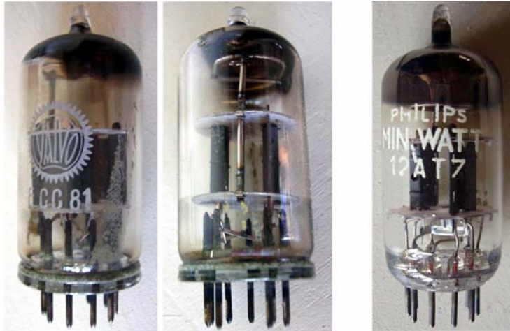
Fig. 4 - Two images of an early glazed version of European ECC81 /12AT7. Although branded as Valvo, its short code Y4B printed on the base suggests a British Mullard production, at least up to pumping. The last sample is a more recent miniature Philips 12AT7.
