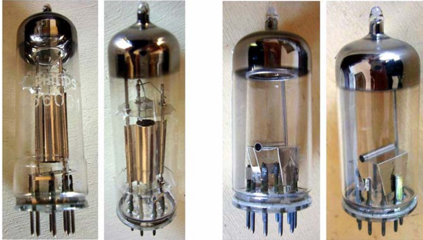
Fig. 7 - The two photos on the left show a temperature limited diode 5601 , intended to be used as feedback sensor in AC voltage stabilizer circuits. On the right we see another temperature limited diode, the K81A , intended for use as noise generator. Both were assembled with base glazing technique.
