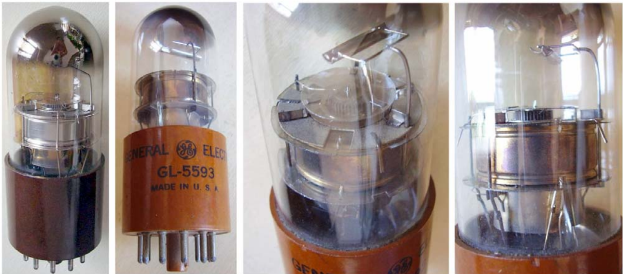
Fig. 1 - General Electric registered two devices, the 2H21 and the 5593. Here the photos of the two phasitrons with details of the electrode structure inside.
