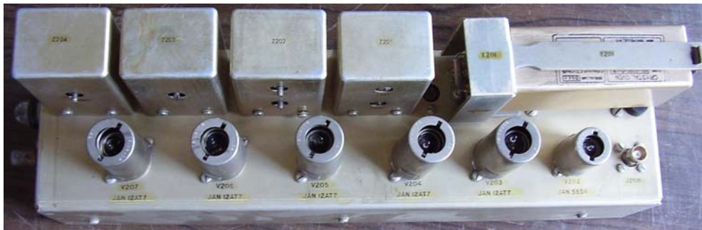
Fig. 2 - The 10 kHz generator subchassis. The 1.250 kHz crystal reference is in the oven at top right.
