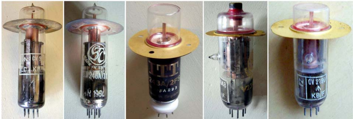
Fig. 1.4 - Some samples of British Heil oscillators. From left, CV228 and its alternate selection CV485 , CV5463 . The last two photos are of CV5048 and CV2190 .
