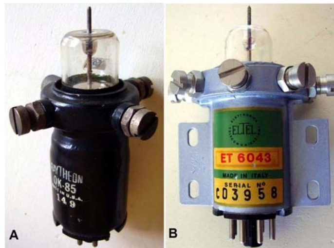
Fig. 8 - Two Raytheon packaged klystron oscillators. Both QK-85 and 6043 were variants of 2K28, with factory installed resonator. The sample in the right photo was made by EITel, formerly ELSI which in the early sixties was a qualified Raytheon plant in Palermo, Italy.
