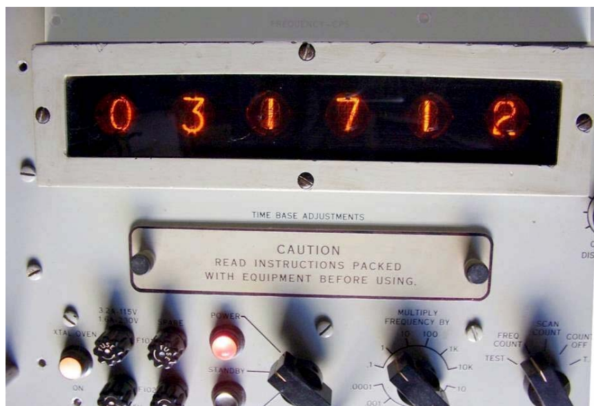
FR-114/U digital frequency meter using trochotron decade counters. Click on image for more information.
