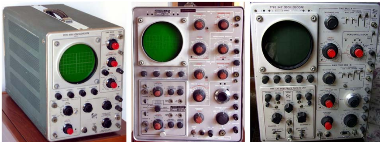
Fig. 05 - Tektronix oscilloscopes. Left, a small 515A intended for service. The Lavoie LA-265 was a clone of the Tektronix 545: dual time base and distributed gain vertical amplifier, rated for 30 MHz minimum bandwidth. The third oscilloscope is one of the 547 used by the late Prof. Angelo Luciano, the one who made so many people understand the secrets of electronics. The instrument had been partially cannibalized, but today the restoration is almost complete.
