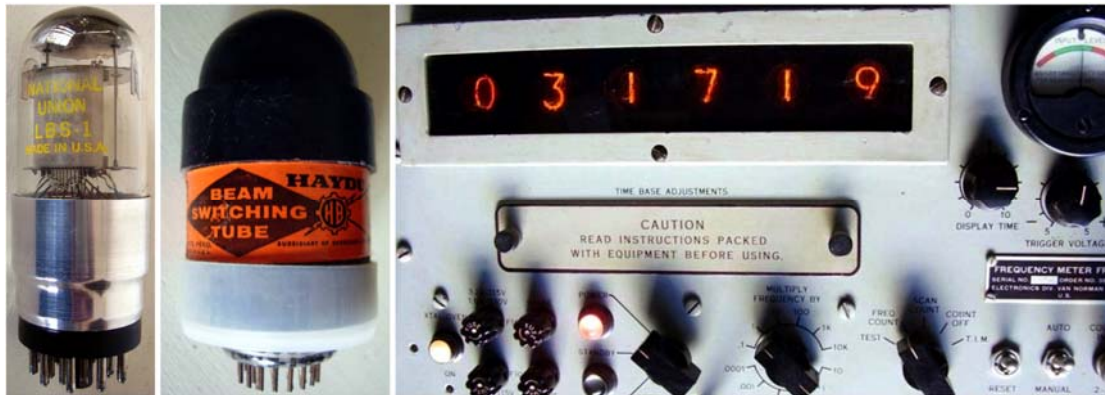
Fig. 04 - Left, a beam switch selector LBS-1 , forerunner of the trochotron, and a sample of the first external magnet 6700 trochotron manufactured by Haydu Brothers, on the design carried out at Burroughs. Right, a digital frequency meter, the FR-114/U , based upon six trochotron counters driving 6844 Nixie readouts.
