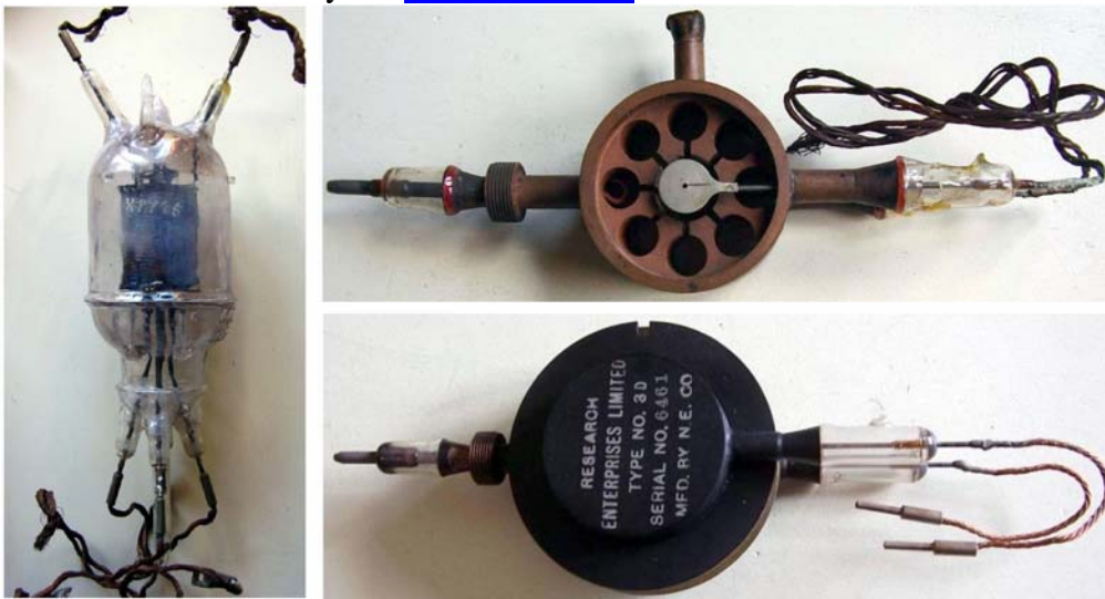
Fig. 02 - Left, a sample of silica valve, the NT57 , used in the early operational British sets in the second half of the thirties. Top right the first laboratory prototype of the eight-cavity E1189 magnetron. It was used at GEC by E.C.S. Megaw to characterize his low magnetic field and low profile pulse design, a variant to the CW prototype devised by Randall and Boot at Birmingham. The sealed E1189 sample no. 12 was brought to America and Canada by the Tizard Mission, originating there countless copies and variants. Bottom right, a REL 3D , Canadian copy of the E1189, made by Northern Electric. Just the accidental discovery of the E1189 prototype, coming from a warehouse of the disappeared GEC, allowed us to reconstruct the history of the development of the British magnetron .
