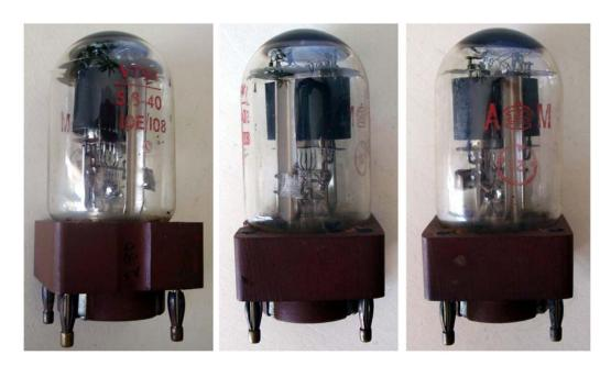
Transmitting triode mounted on low-loss L4 British base. Filamentary cathode.
