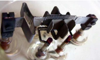
Almost certainly TS6 was the biggest doorknob style UHF triode ever made. It was designed during WWII by German GEMA for the marine radar Seetakt operating around 400 MHz. Also used in some Freya sets. It replaced <u>TS1</u> and <u>TS1A</u> which were similar to WE <u>316A</u>. Rugged electrode structure to withstand heavy shocks and vibrations due to heavy gun firing aboard of battleships. Filamentary thoriated-tungsten cathode formed by eight wires in parallel for higher emission.
