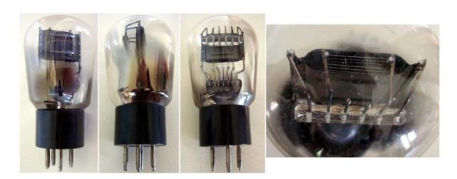
.No info found on this triode. We know from the residual writings on the bulb that it was made by Zenith and its filament operates at 4 volts, 0.25 amps.
