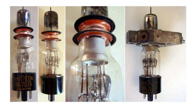
External cavity reflex klystron, intended for use as local oscillator in radar receivers operating around 3 GHz. The 707A was the early reflex klystron developed by Western Electric capable of operation at considerably low voltage, around 300 volts. The corresponding British oscillator, the Sutton tube, required resonator voltages in the order of 1500 volts, with considerable insulation problems in airborne equipment. Early samples delivered by the late 1941, volume production from early 1942.
