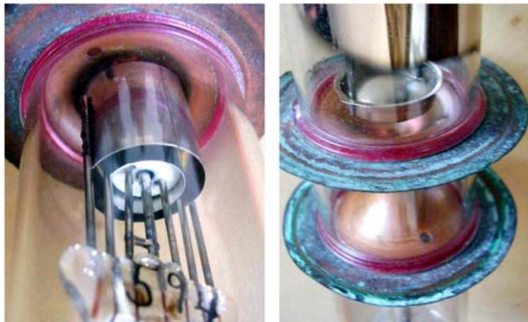
Detailed views of the electron gun subassembly and of the cup-shaped reflector, very similar to those in the [Sutton tube](#). Below a partially disassembled 8B.
