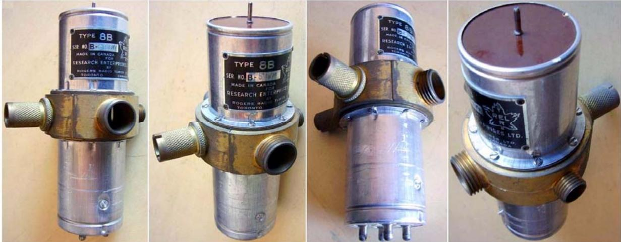
Very few information on this Canadian klystron, also known as RT66. Sibley lists four frequency variants from 8A to 8D. Presumably two of them matched the frequency of [3C](#) and [3D](#) magnetrons, equivalent to British CV38 and [NT98](#). The shape of the two cavity terminating horns and the cup shaped reflector suggest that it was directly derived from the original British '[Sutton tube](#)'. See also draft at page 79 of *Metres to Microwaves*, Callick.
