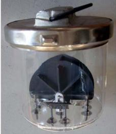
UHF power triode, designed to operate at frequencies up to 600 MHz. Oxide coated unipotential cathode, finned anode. Two tubes plate keyed in push-pull were used in the transmitter section of the FuG 200 Hoentwiel airborne radar, generating 30 kW pulses, 2 us wide at 525 to 575 MHz.
