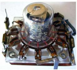
This is a developmental prototype of the secondary-emission orbital beam VHF amplifier, known as VT-128 or <u>1630</u>. In this sample, complete with its custom base, the twelve radial pins are equally spaced.
