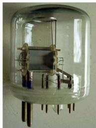
Double tetrode designed to operate as amplifier, tripler or oscillator in the UHF region. Special loctal base with separate anode pins.
