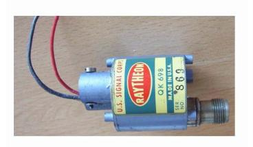
Low power pulse magnetron for beacons. Integral magnet, coaxial output.
