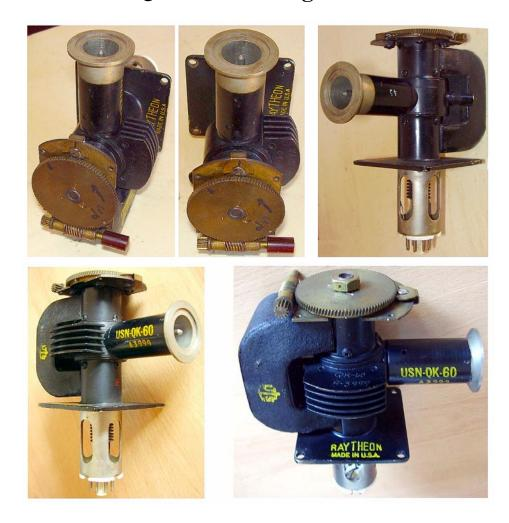
50-70 W pulse magnetron for radar jammers. Integral magnet, coaxial output. Probably derived from the CM16B prototype described in 'Microwave Magnetrons', by George B. Collins, MIT Rad. Lab. Series, Vol.6.
