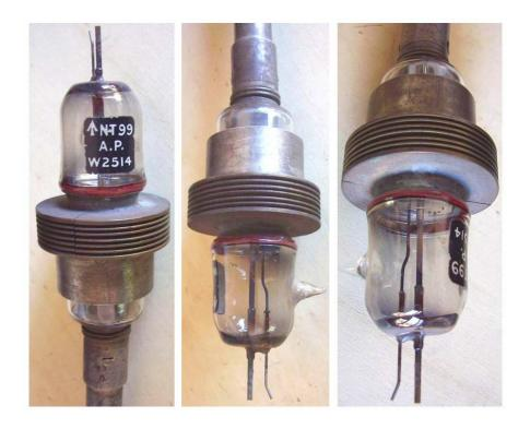
Micropup power triode, also referenced to as Admiralty Pattern W2514. Full emission selection was approved as CV1256, low emission units being approved as CV199.
