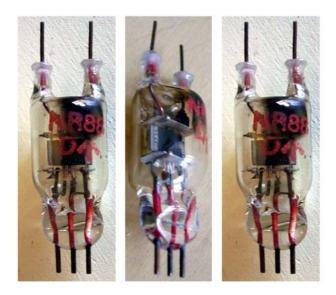
Miniature UHF triode, capable of operation as oscillator up to 600 MHz. 50 mm approximate body length.
