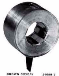
Fig. 4. — Oscillation system of a turbator. The resonator is built of very heat resistant and well degassed metal.
