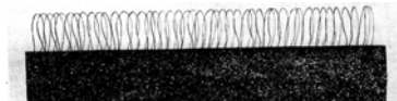
- Typical construction of grid in a doorknob triode. Small tungsten loops are welded to a supporting plate
